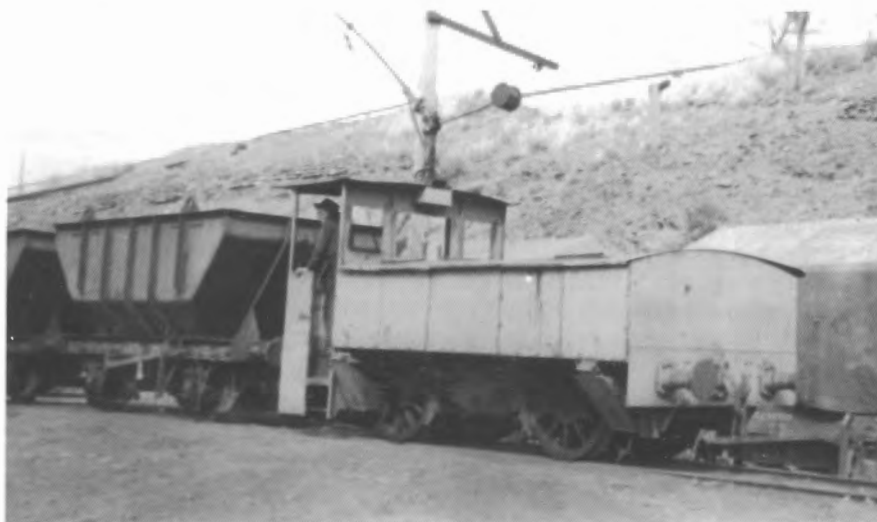
Mt Morgan Mine, 13th August 1957: 3ft 6ins gauge electric built using QR B13 wheelsets, shunting coal on Linda level. Photo: John Knowles
