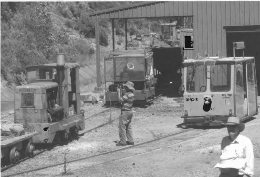
Top: McConnell Dowell's F&M Baldwin 4wDH hydrostatic rack locomotive 040/156 (FMB12TRA-295 of 1995) stopped for repairs at the Bogong headrace access tunnel on 16 November 2008.
