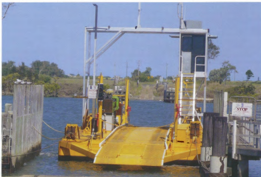
Cane bins are piggy-backed on semi-trailers between the Bingera and Millaquin systems across the Burnett River at Fairymead using this ferry. 6 November 2008.
