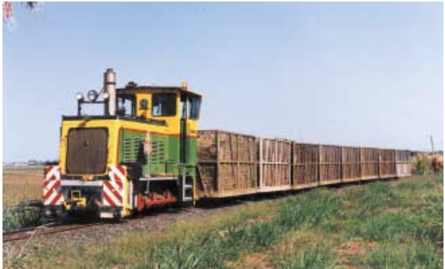
Farleigh Mill's Clyde 0-6-0DH CONNINGSBY (61-232 of 1961) has just crossed the Miclere catch-points with the last eight bins of cane from Dumbleton for the 1999 season. The fireman makes the short walk back to the loco for the run up to the mill. 20 November 1999. Photo: Andy Roberts
