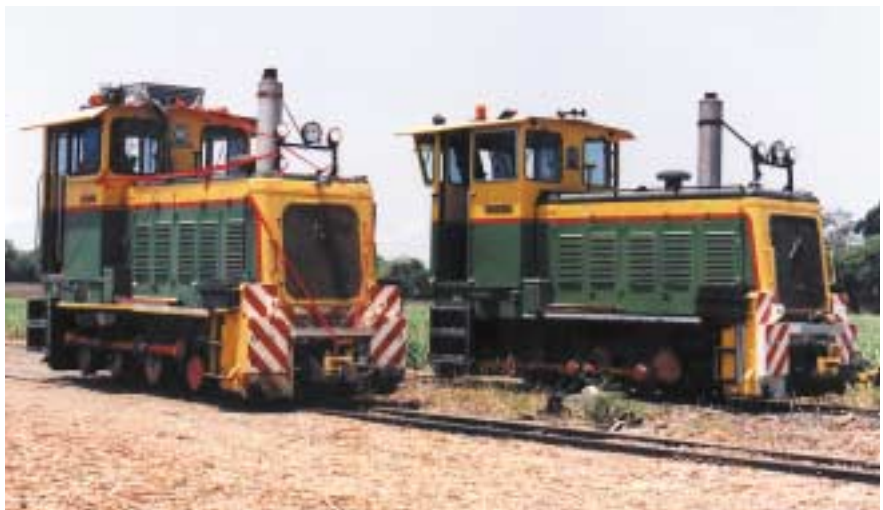
Farleigh Mill's Clyde 0-6-0DH ST.HELENS (61-234 of 1961), decorated to celebrate the end of the season, has just delivered empty bins while CONNINGSBY (61-232 of 1961) is picking up fulls at Calen on 20 November 1999. These locos, both in the Mackay Sugar corporate livery, provide an interesting study in differences in cabs, paint schemes and other details. Such variations mean that mill personnel are easily able to recognise different locos at a distance. Photo: Andy Roberts
