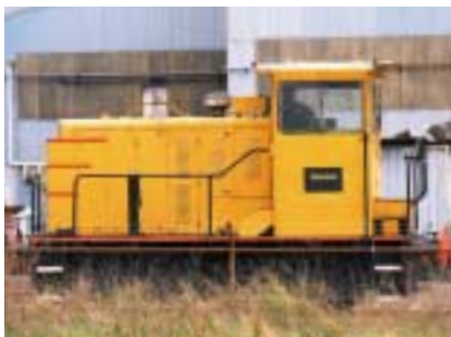
Comsteel's little Goninan 4wDE (030 of 1972) on 12 February 2000. This rigid wheelbase loco gives the appearance of being a cut-down version of the more familiar bogie type. Photo: Brad Peardon
