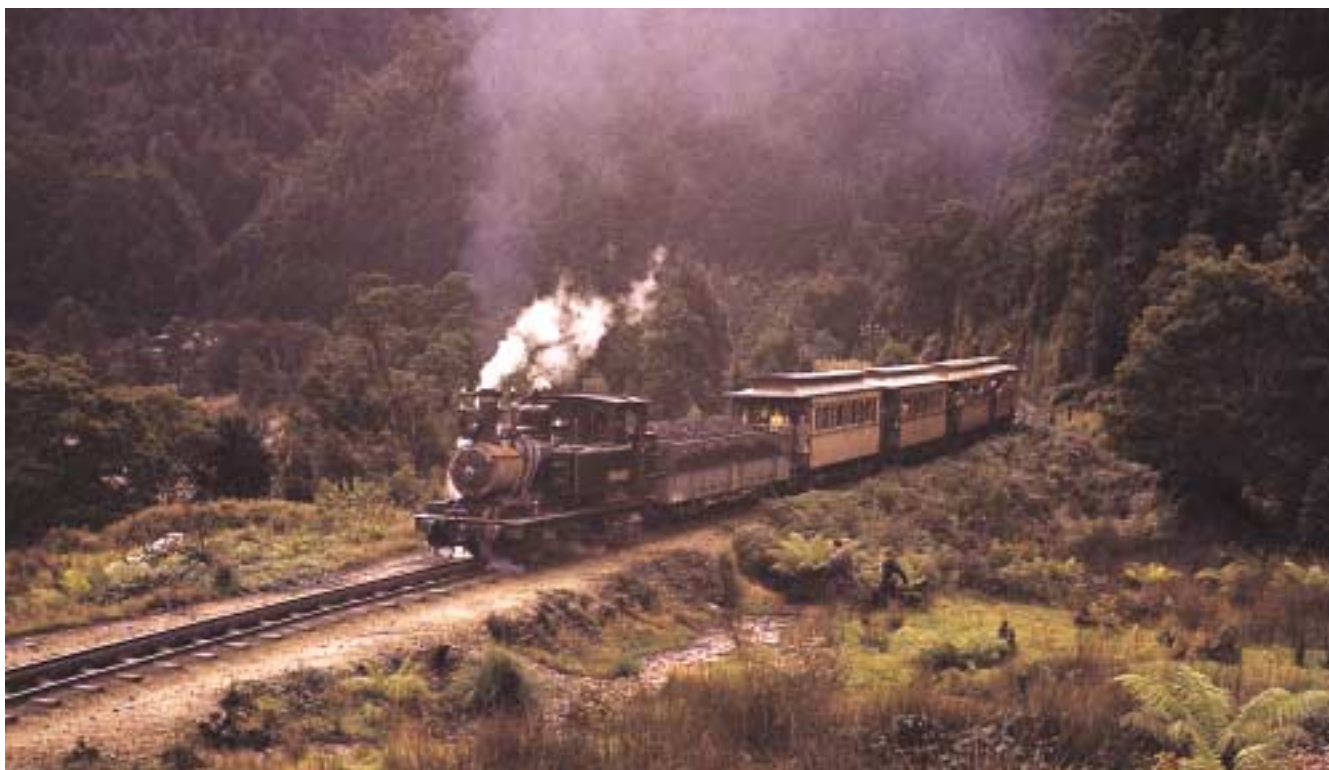
Abt No.3 (Dübs 3730/1899) climbs the rack section out of Dubbil Barrill with a passenger train, on 16 April, 1960. Photo: Peter Charrett
