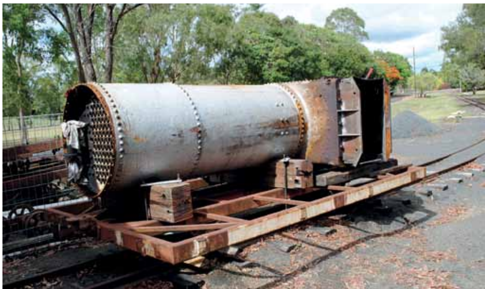
The boiler from the Bundaberg Fowler 0-4-2T locomotive (3 of 1952) on a wagon outside the depot in the North Bundaberg Botanical Gardens awaiting the attention of a specialist welder.
