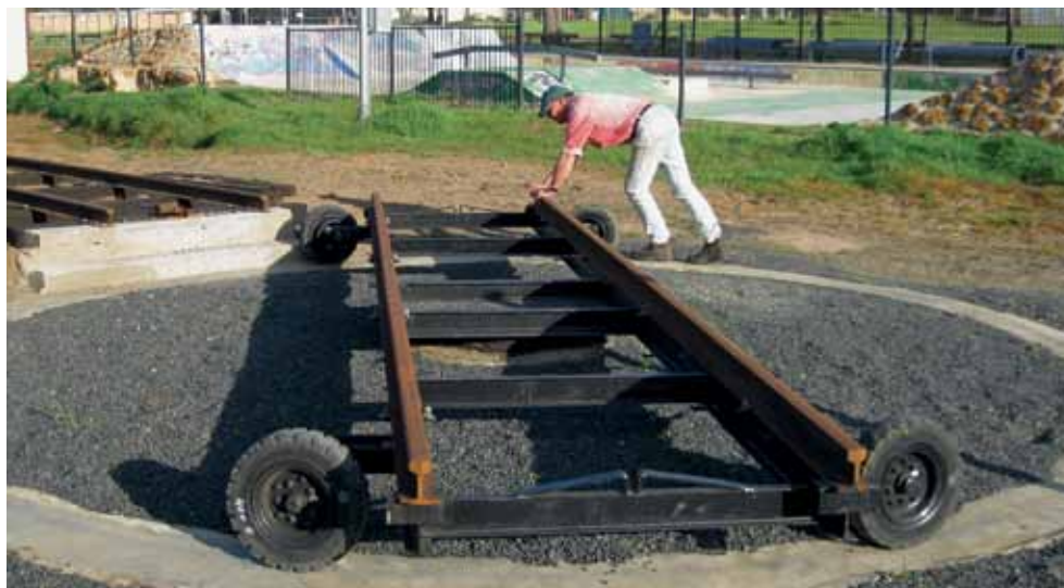
Ned Radford demonstrates the turntable installed at Kojonup on 1 September 2011. It utilises the turntable from one of the former Perth Zoo road-train carriages and will be used to turn the locomotive following its conversion to rail operation. Photo: Bob McKillop
