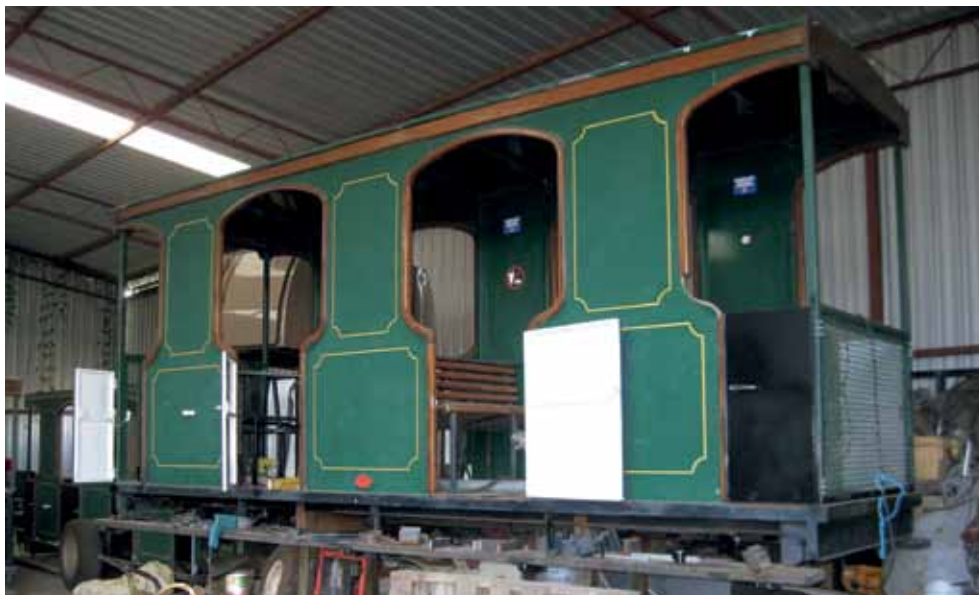
One of the three former Perth Zoo road train carriages undergoing restoration and conversion to rail operation at John Lewis' workshop in Kojonup on 1 September 2011. Photo: Bob McKillop
