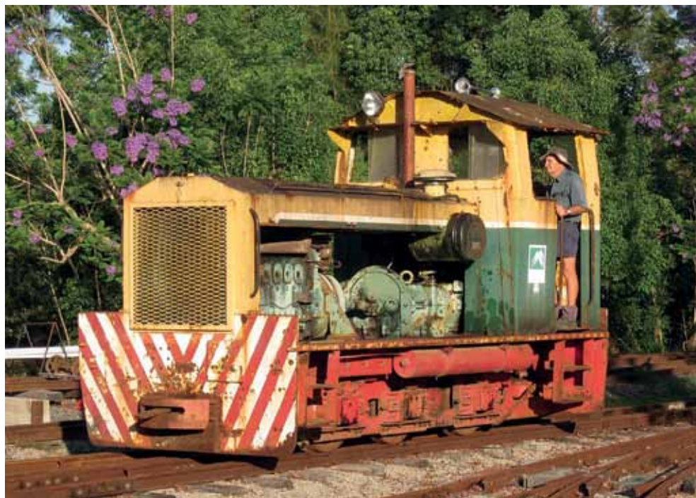
The ex-Marian Mill 6wDM NETHERDALE (Bundaberg Foundry 13 of 1954) being given a trial run on the Durundur Railway on 12 November 2011 prior to overhaul as a back-up locomotive.
