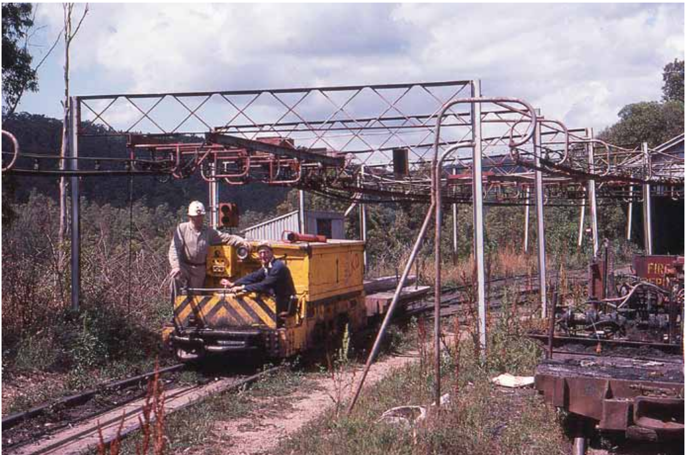
Out in the light of day, one of the Stockrington battery locomotives is posed for a photograph on the weed-infested pit top trackwork in January 1978. The elaborate overhead support structures are associated with the mine's unique over-running current collection system used by the larger, trolley-wire locomotives.
