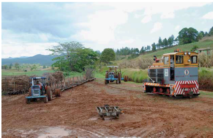
Owing to inadequate siding infrastructure amongst other things, overlanding of empty cane trucks has become common practice in Fiji and in this scene on 20 October, Labasa Mill Clyde 0-6-ODH 9 (62-270 of 1962) stands by while tractors yank their shares of trucks out of its rake of empties at Vuliaki. Photo: John Browning
