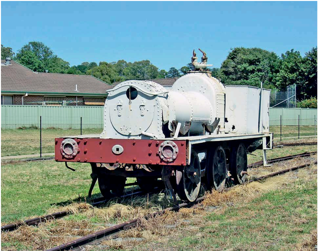
The remains of locomotive 530 awaiting further restoration at the Yass Town Railway Museum, December 9, 2012. Important parts missing are the stovepipe chimney, the circular saddle tank, and the rounded cabin and roof. Source: Peter Crabb
