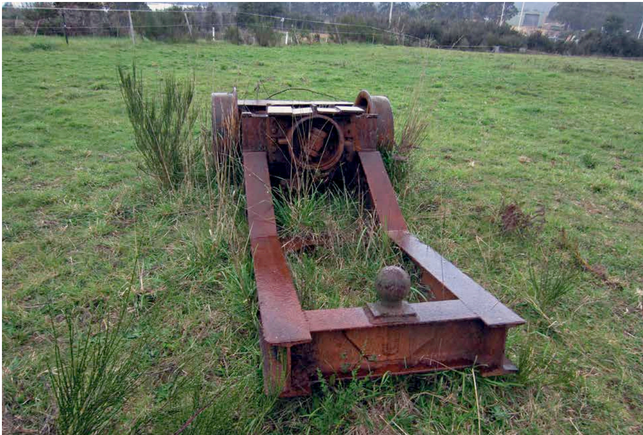
A front-end view of the 'mystery frame' or assembly, as it lay upside in a paddock about 250 metres from the former Raminea Mill site. It had been moved there during a clean-up of the mill precinct; it is understood that many other mill artefacts were disposed of elsewhere during the clean-up. Note the cranked stringers, and the large (120 mm dia) tow-ball which, in the normal (inverted) orientation, apparently sat into a housing in the ex-Byers bogie, thus providing The Caterpillar's with leading articulated support. Photo: JS Clennett Sept 2016
