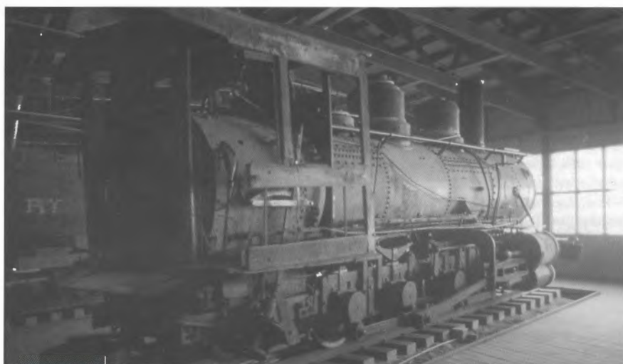
Klondike Mines Railway No.3 - Baldwin Vauclain compound 2-8-0 locomotive, B/No. 16456 of 1899 at "The Locomotive Shelter", Dawson City Museum, Yukon Territory in July 2001. It was built for the White Pass & Yukon Route, originally their No.7, and later renumbered 57. They sold it to the KMR in 1906. Photo: Frank Stamford
