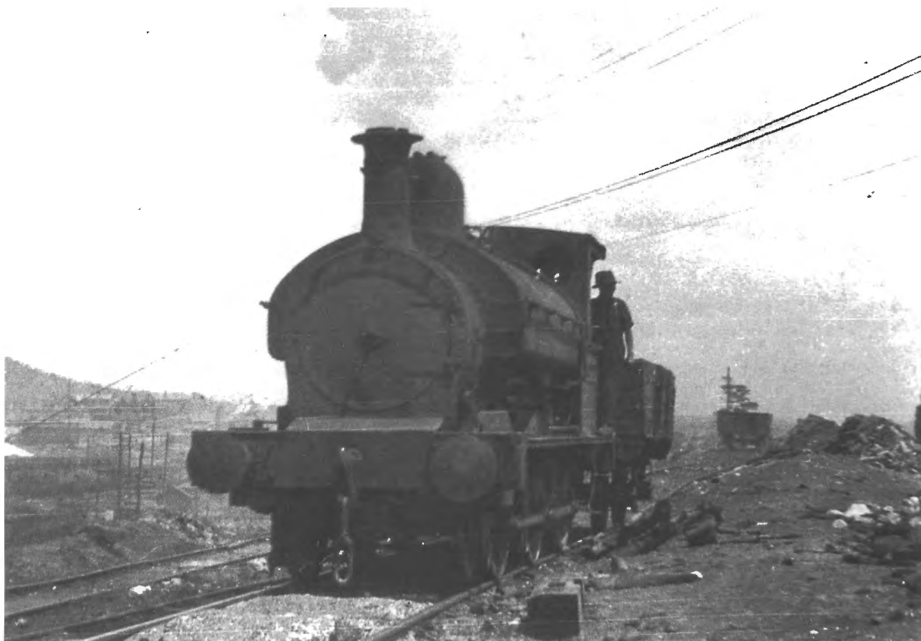
Beyer Peacock 0-6-0ST KOALA (1418 of 1873) seen here shunting in 1927, was used for coal and coke haulage around the coke ovens at Lithgow. Transferred to the new Port Kembla works in 1932, it was found sufficiently useful to be given a new boiler six years later. KOALA was finally retired in October 1955, at the ripe old age of 82.
