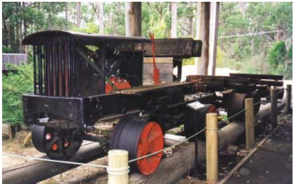
This 4-wheel IC-powered logging tractor is on display at the Bush Mill complex at Port Arthur, Tasmania. Automotive-type leaf springs are visible between the wheels and frame. Photo: Wal Lane
