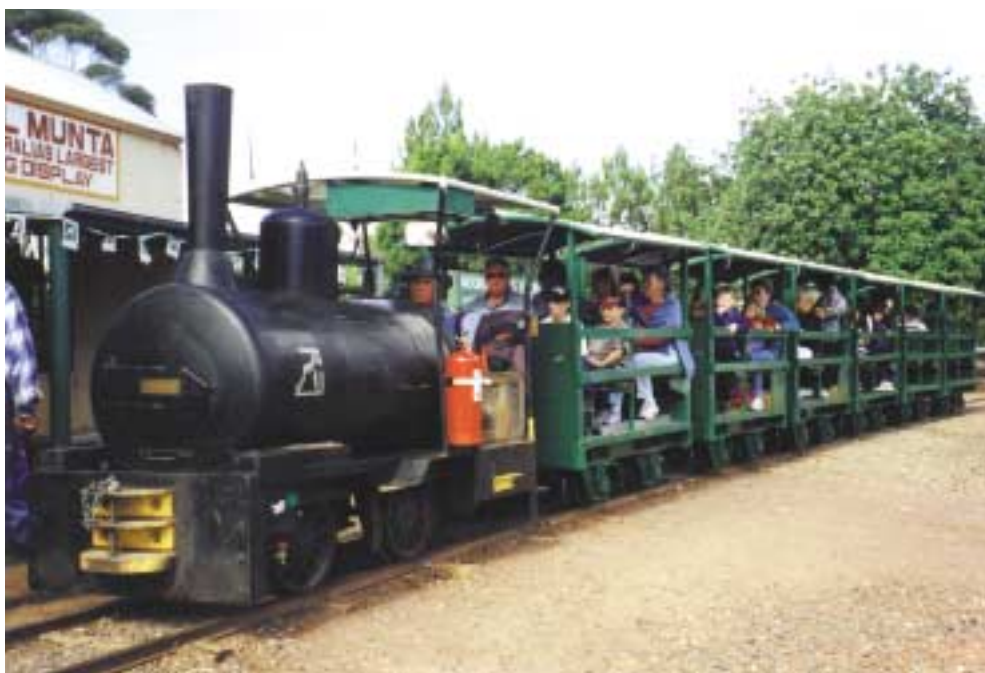
The 4wDM steam outline locomotive hauls a well-patronised train of visitors at the National Trust Moonta Museum & Tourist Tramway. The locomotive was built on the frames of a loco from the Adelaide Zoo and has been modelled after the 0-4-0WT that once operated at Moonta under the local name of Captain Hancock's Pig. Photo: L Brandt
