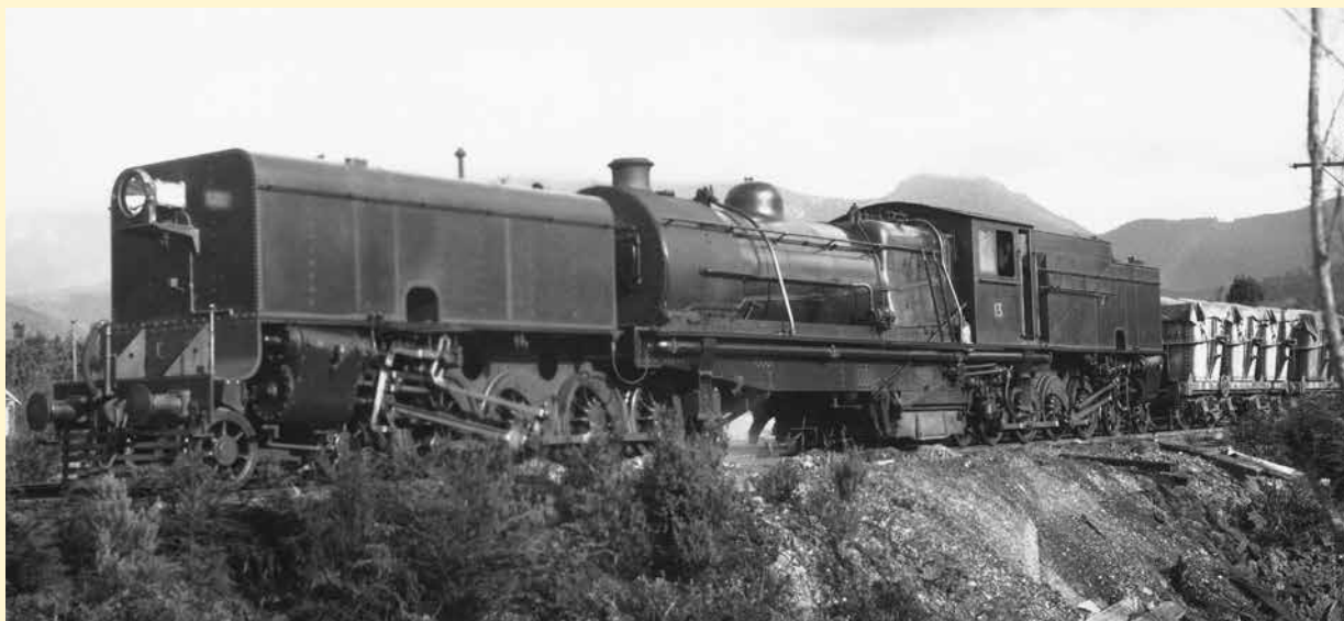
Emu Bay Railway No.13 (BP 6581/1929) on No.5 train running special, stationed at Primrose 3 Feb 1937. The 3ft 6in-gauge EBR purchased three of these impressive Garratts in 1929. With a tractive effort of over 42,600 lbs (@ 85%) and weighing around 133 tons, they were well suited for the heavy ore traffic on the Tasmanian West Coast. The design was a copy of the metre-gauge Kenya-Uganda Railway EC-class of 1926 (the pioneering 4-8-2+2-8-4 Garratts), the only real differences being the gauge and the EBR locos carrying 1000 gallons more water and a slightly higher boiler pressure. No.13 was withdrawn and scrapped in 1961. Photo: J.L.N. Southern
