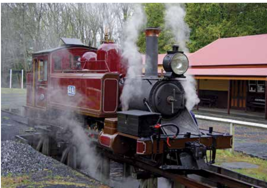
A spectacularly restored 12A at Gembrook on its third day back in regular traffic after an extensive reconstruction. A post restoration feature is "decorative" glued on rivet heads applied to the new, welded side tanks. Photo: Graeme Daniel 10/13
