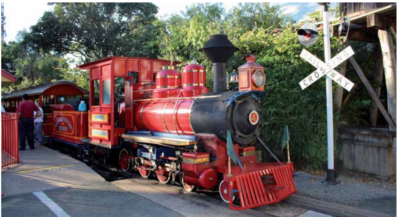
Pictured at Dreamworld's Central Park station two months prior to replacement by the new diesel outline loco, REG. COULTER (Baldwin 4-6-0 45215 of 1917) sits waiting for the next departure. Photo: Mark Gough 10/8/13
