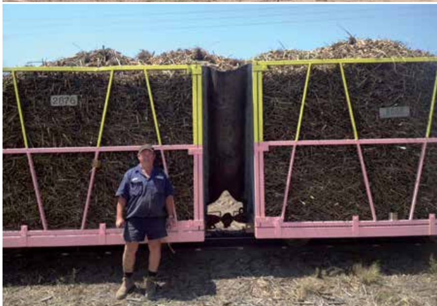
Top: Tully Mill's new Chinese-supplied spot tamper, 23 September 2013. Photo: Luke Horniblow Centre: The newest addition to Tully Mill's fleet of rebuilt Walkers DH-class B-B DH locomotives, TULLY-3 , shunts fulls at Daveson Road, El Arish, on 21 September 2013. Above: Interesting experimental 'corridor connection' between two Invicta Mill bins, designed to accommodate the needs of elevator tipper loading and increase per-bin tonnages, September 2013. Photo: Canegrowers Budekin Limited
