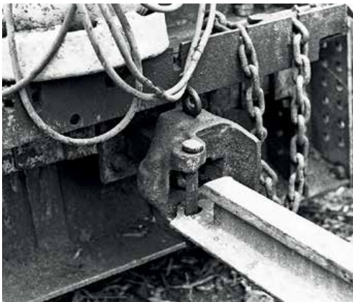
Left and right: Close-up views of the coupling between the locomotive and rail trolley – definitely the creation of a fully-qualified bush mechanic!
