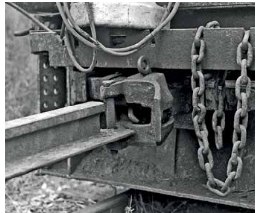
Left and right: Close-up views of the coupling between the locomotive and rail trolley – definitely the creation of a fully-qualified bush mechanic!
