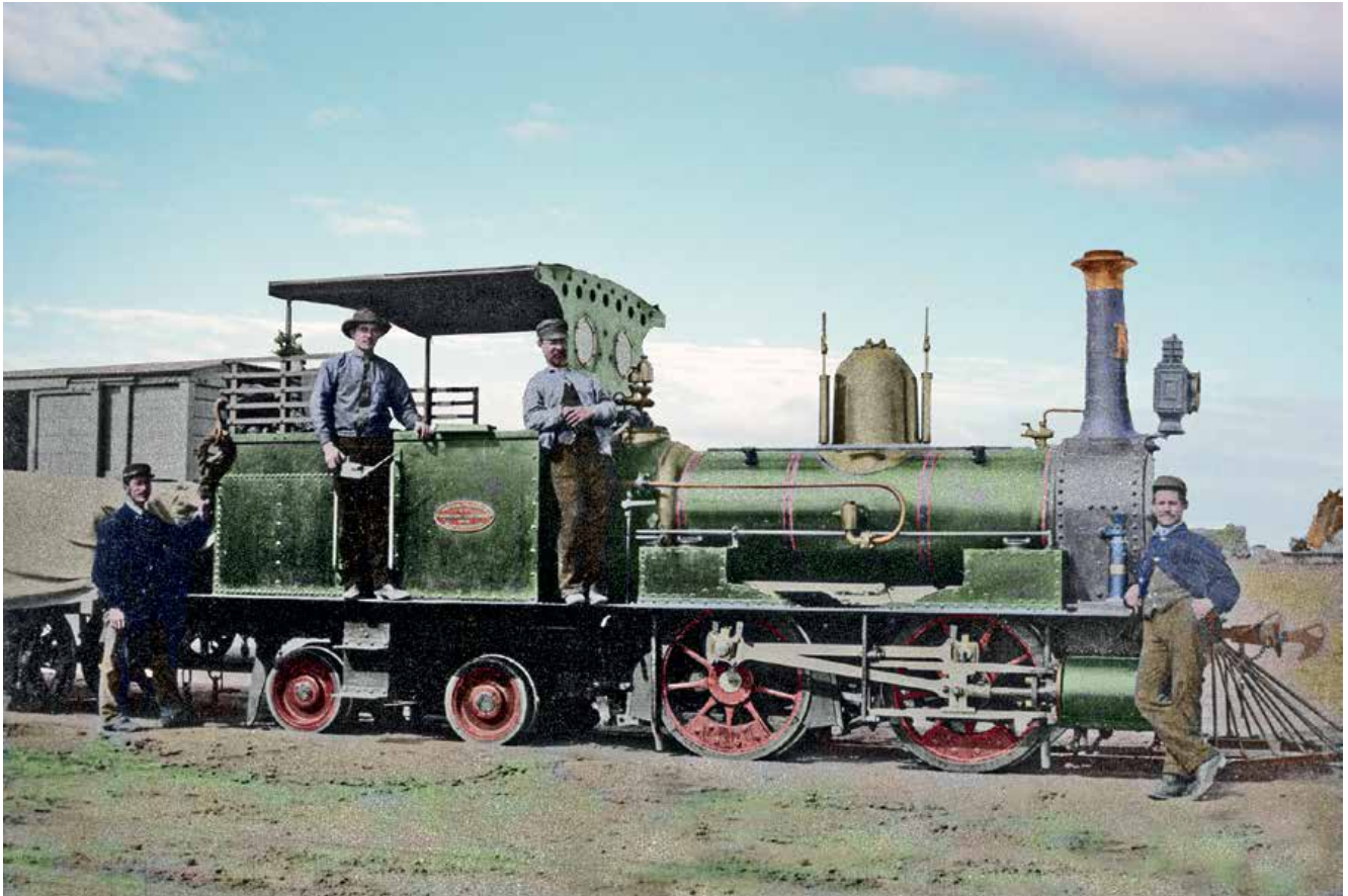
South Australian V class 0-4-4BT locomotive No.10 or 12 in near new condition. The location is unknown, but is most probably on the Kingston – Naracoorte railway, or at Port Augusta. The tinting is based on the Beyer Peacock livery when the locomotives were new.
