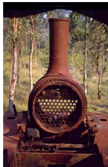
No.530; a view the cab of the smokebox, front tubeplate and part of the motion, Kalingo, January 1973. Photo: Shane O'Neil
