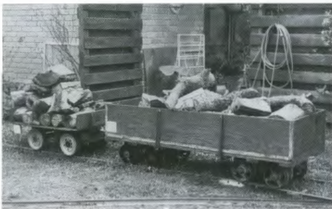
A loaded firewood train parked on the siding near the wood box. The four-wheel wagon has brake drum wheels, while the bogie wagon has wheels taken from old mine skips.
