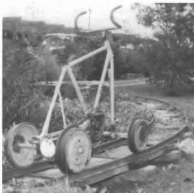
This 15in gauge 'pushbike' utilised old car brake drums as wheels, and carried a white 'end of train' disk on the rear.
