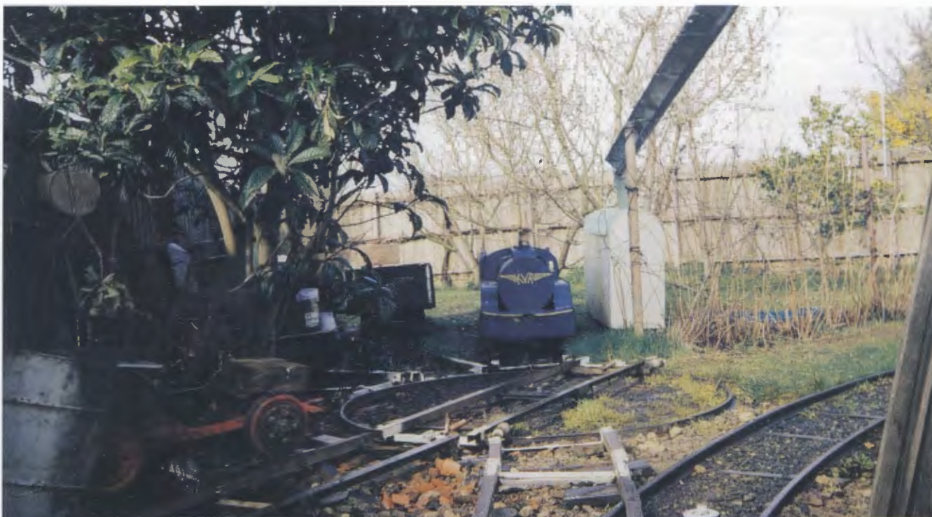
The turntable and surrounds, seen in August 1989. On the left is the electric Trolley, with the 4-wheel truck behind. Next is the bogie wagon and, in the centre, the 4-6-0 locomotive. The 'layover' points in the foreground are set for the turntable.
